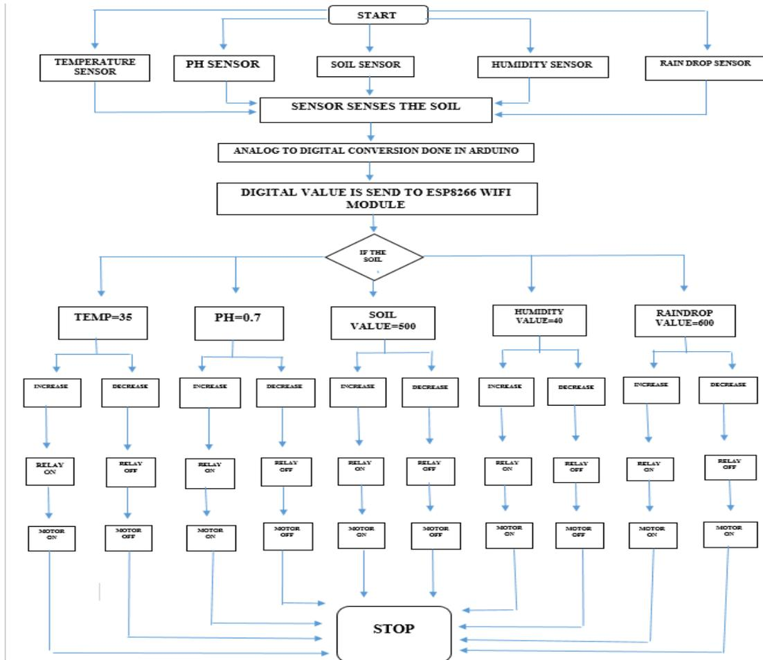
Figure 3.3: Working Model of Automated Irrigation System
