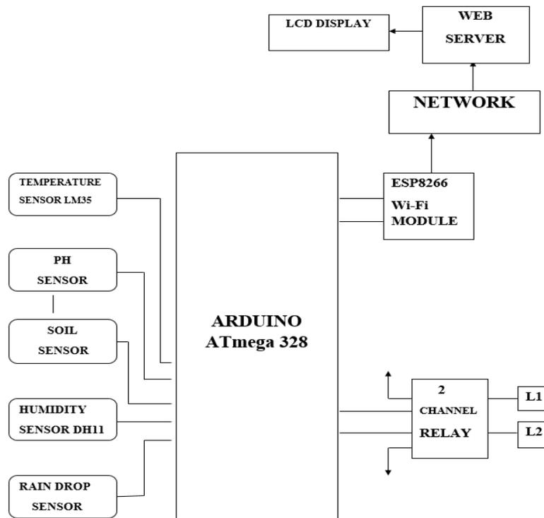
**Figure 3.2: Circuit Diagram of ARDUINO ATmega 328**
