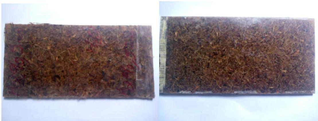
**Figure 2** Fabricated Oil Palm fiber Composite
