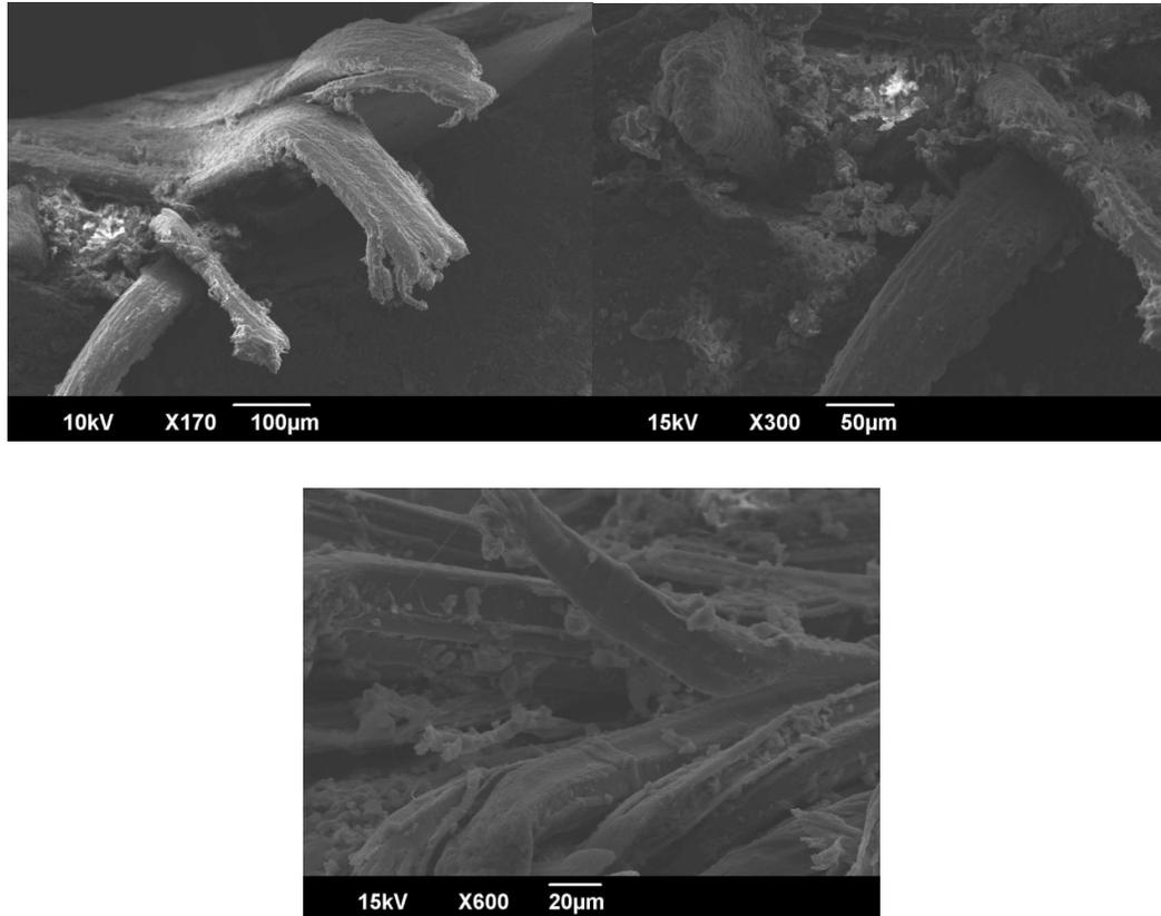
**Figure 4** SEM Micrographs of Oil Palm Fiber Composite
